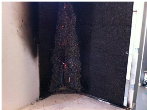
Figure 7. Cork panel after the SBI test.
