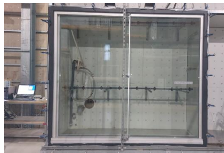
Figure 8. Aluminium minimal window during wind resistance test
