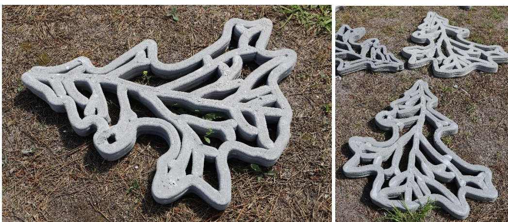
Figure 2. Extruded bionic shape specimens based on grey cement — CEM I 42,5R.
