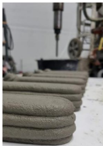
Figure 1. Extruded specimens for compression test based on grey cement — CEM I 42,5R.
