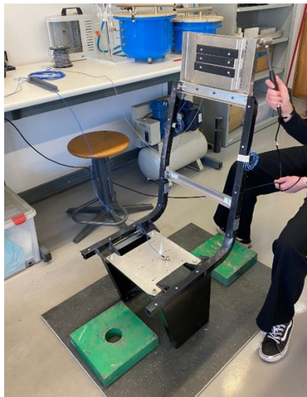
Figure 2. Vibration Tests of the prototype seat skeleton.
