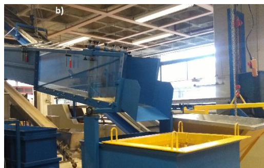
Figure 2. a) Scheme of the channel employed at the University of Trento to analyse the driftwood transport, with the positions of the three cameras and the reference points for the measurements; b) view of the tilting flume at the University of Lisbon.
