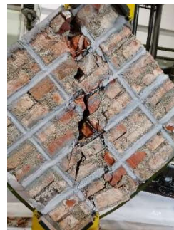
Diagonal compression (Reinforced)
