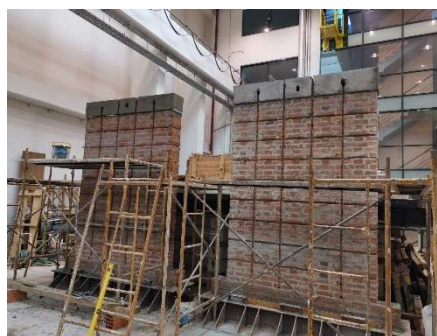
Full-scale masonry walls (shaking table)
