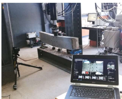
Flexural behavior of eco-efficient and ultra-high durability concrete beams: test set-up (left) and load-displacement relation (right).
