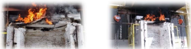
General views of a fire resistance tests on a foam-filled sandwich panels.
