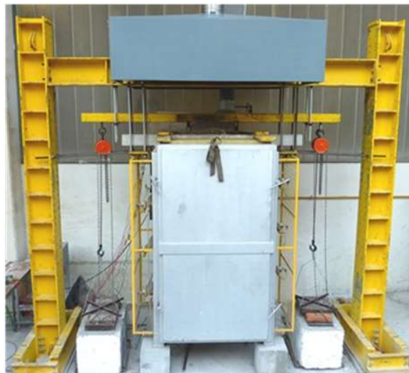
Fire resistance tests setup.
