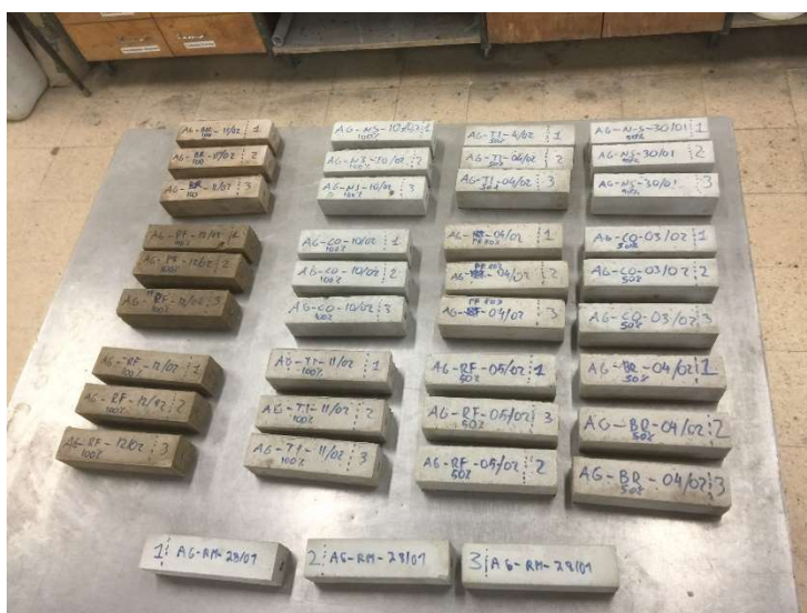
Samples of the mortar, produced with CDW' rubbles.
