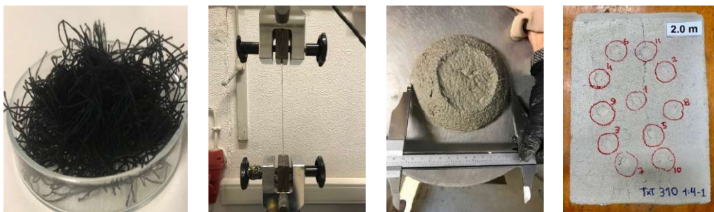
Recycled fibres waste incorporated in rendering mortars.
