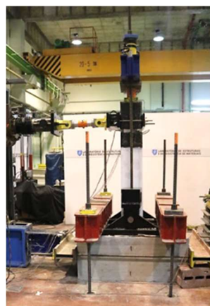
Overview of the test setup adopted to evaluate the behaviour of GFRP-reinforced concrete columns subjected to different loading scenarios.
