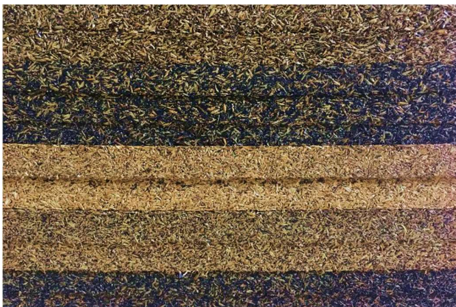
Samples of the composite materials, made from rice husk, expanded cork and recycled rubber.
