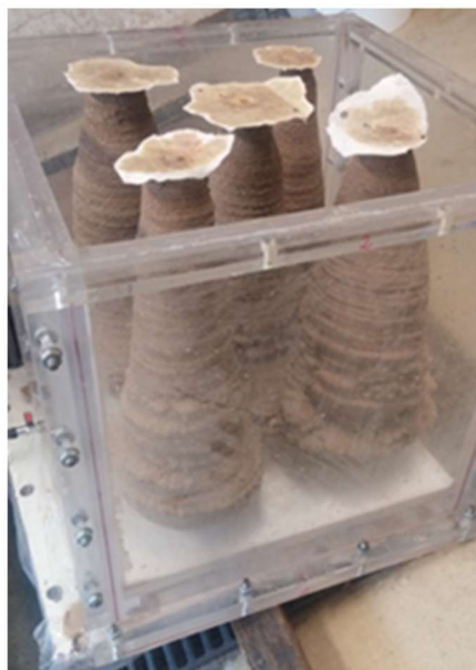
Sand box design (left) and columns of sand-resin mixture after injection (right).
