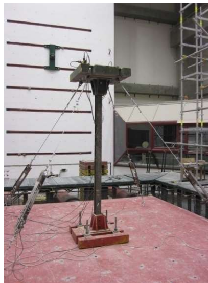
Shaking table test set-up.
