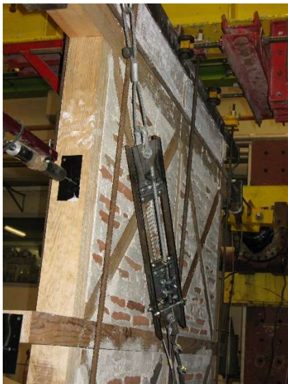
Wall reinforced with superelastic damper.
