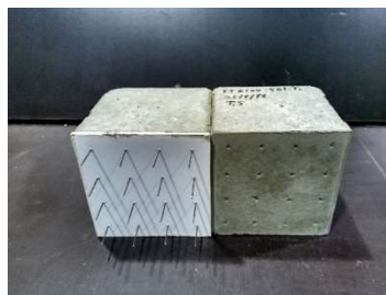
Fibre/matrix interface: bond stress-slipping curve (left) and specimen configuration after the test (right).
