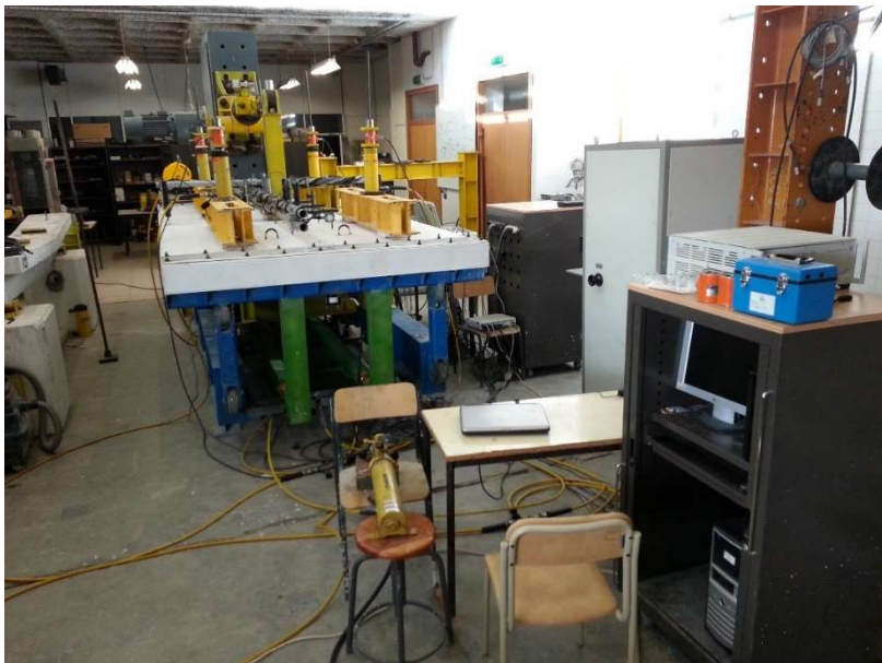
View of the test setup and the data acquisition equipment for the cyclic tests of SFRC flat slabs under horizontal cyclic loading.
