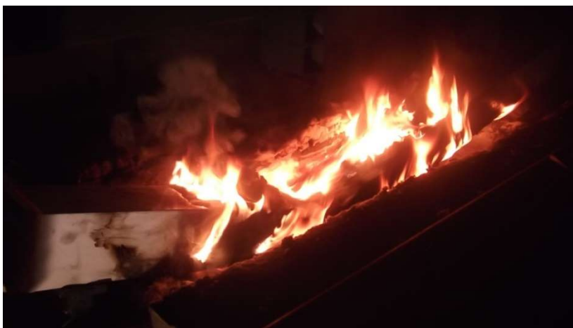
Fire resistance tests performed on GFRP tubular beams.
