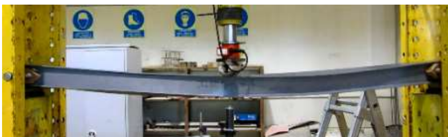
Structural beam testing, removed from service conditions, after 15 years of ageing next to the sea.
