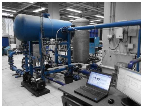
Test-Hydro pipe-rig for testing small-power reaction turbomachines in both transient and steady state conditions, assembled at the Hydraulics and Water Resources Laboratory of IST.
