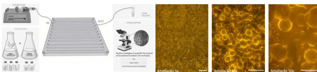
Figure 1. Scheme of the microfluidic device and preliminary results showing calcite particles.
