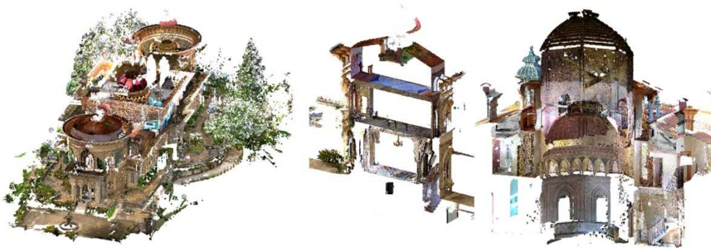
Preliminary point cloud in Autodesk Recap software of the Case Study - Monserrate Palace, Sintra.
