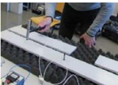
Dynamic characterization of free-supported FRP-Beam
