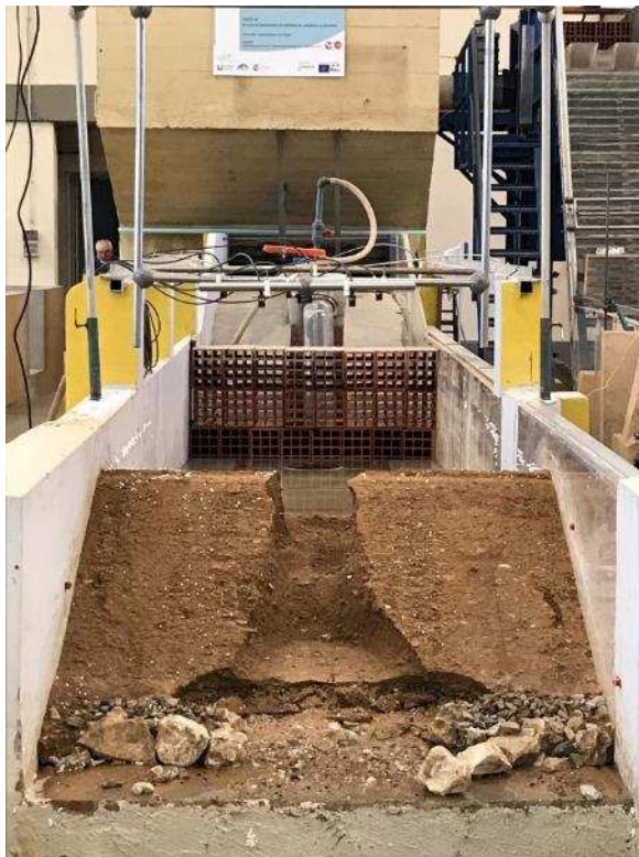
Dam breach by overtopping. Experimental test.
