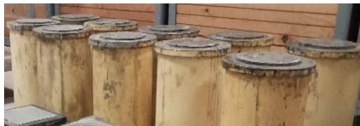
Figure 3. Specimens expansion inside the moulds.
