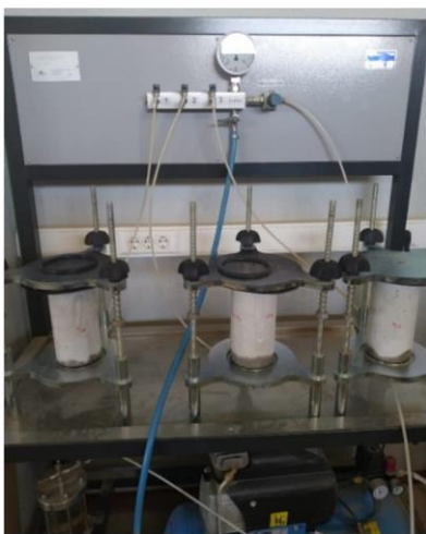
Figure 1. a) Water penetration under pressure test; b) penetration depth in a recycled concrete specimen with treated surface with a bioproduct produced based on mixed microbial cultures from pinewood waste [Serrano-González et al., 2021 - https://doi.org/10.3390/ma14216545 ].
