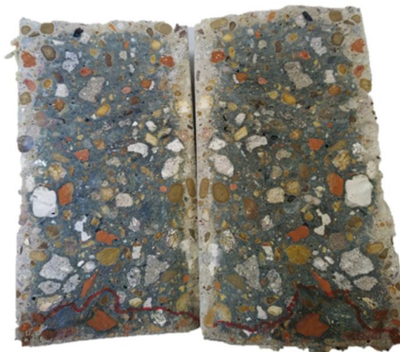
Figure 1. a) Water penetration under pressure test; b) penetration depth in a recycled concrete specimen with treated surface with a bioproduct produced based on mixed microbial cultures from pinewood waste [Serrano-González et al., 2021 - https://doi.org/10.3390/ma14216545 ].
