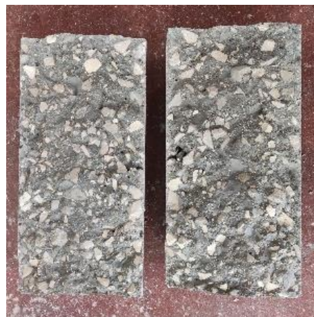
Figure 2. Concrete with partial replacement of Portland cement by reactive MgO.
