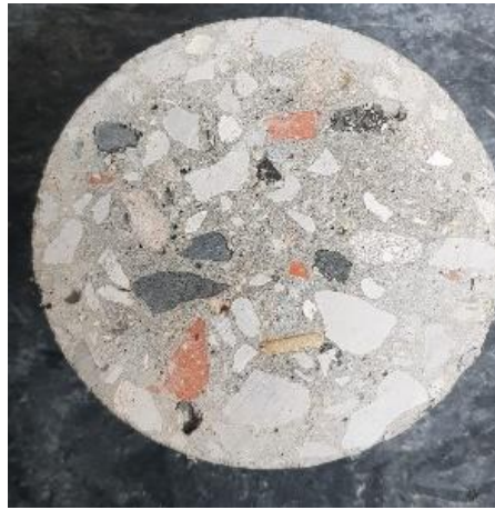
Figure 4. Concrete with partial replacement of natural aggregates by recycled aggregates.
