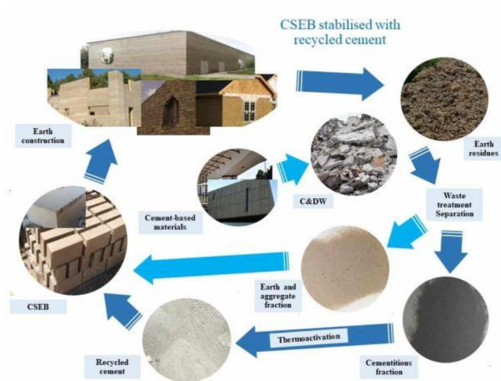
Figure 1. Closing loop of production and recycling of compressed stabilised earth blocks (CSEB) with recycled cement.
