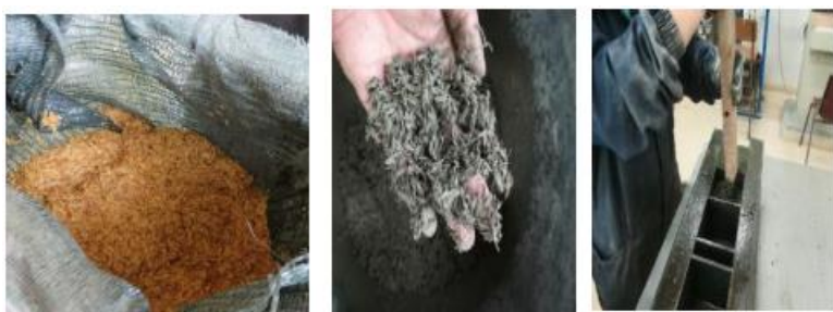
Figure 1. On the left: rice husk; on the centre; mixture at fresh state; on the right: the compactness of the mixture in the mould.
