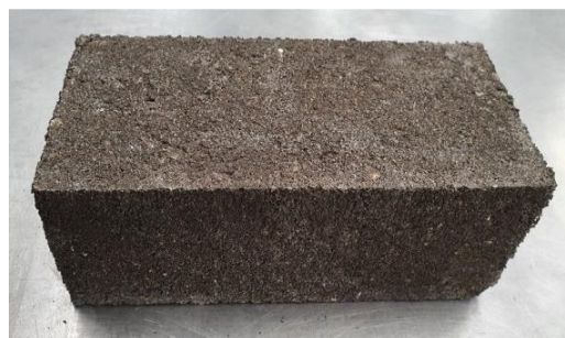
Figure 4. MIBA pavement block according to EN 1338.
