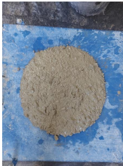
Figure 1. Fresh state tests of recycled aggregate concrete.
