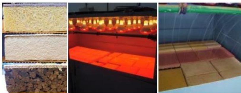
Figure 1. On the left: ETICS solutions; at the centre: Uv-IR irradiation aging tests; on the right: freeze-thaw cycles artificial aging tests.
