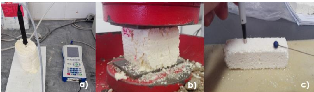
Figure 3. a) General view of the thermal conductivity test setup; b), general view of the compressive strength test setup c) general view of the dynamic elasticity modulus test setup.
