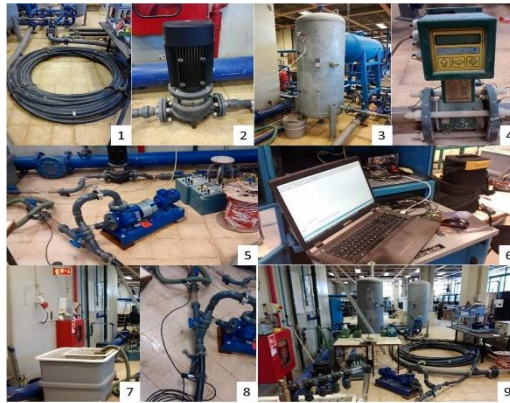
Figure 3. Hydraulic Lab: PAT set-up.
