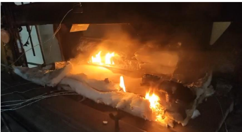
Figure 1. Cork fireproof protection system for windows and doors.
