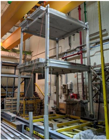
Figure 4. 3D frame shaking table tests.
