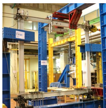
Figure 3. 2D frame sway tests.
