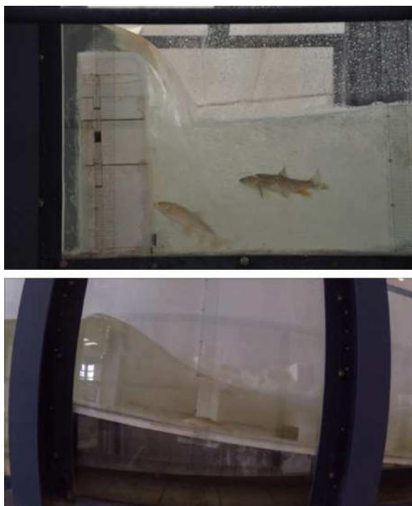
Evaluation of the effect of small dams on the movements of potamodromous cyprinid species: Experimental tests with small weirs with vertical faces (above); and tests with ramped weirs (below).
