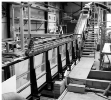
Photo of the physical model with the inclined chute in the background and the stilling basin at the front.
