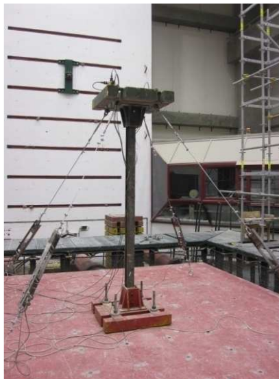
Shaking table test set-up.
