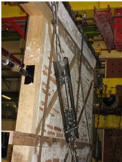
Wall reinforced with superelastic damper.
