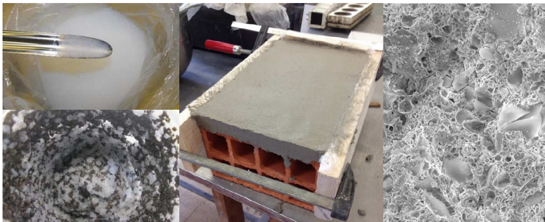
Production, application and microscopic analysis of aerogel-based renders.
